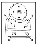
Vehicles with outside power foldaway mirrors have the controls located on the driver door armrest.
